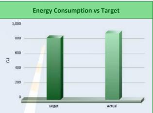
Reliable Controls MACH system calculates a daily target for energy consumption, based on 50% of ASHRAE standard 90.1, adjusted for actual heating and cooling degree days. Standard 90.1 is used to predict the energy consumption of an energy efficient building in our geographical region.
