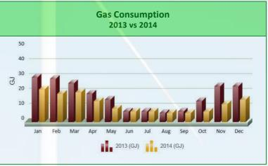
Gas consumption was reduced markedly in 2014, mainly through BAS programming changes that minimized the use of gas for building heat. Most building heat is now supplied by high efficiency electric heat pumps.
